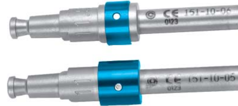
Figure 11 Straight Reamer color-coded bands Full size band indicated full size (11mm), half size band indicates full size plus .5mm (11.5mm)
