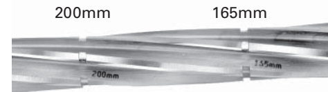
Figure 9 Straight Reamer depth markers
