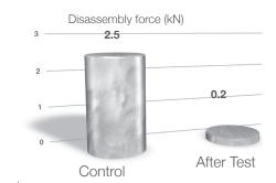
After the test the force needed to disassemble the neck decreased 10 times.
