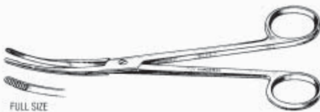
51-6406 Lister Sinus Forceps, curved on flat, screw joint, 18cm.(7in.)
