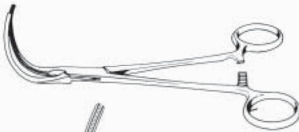
71-2728 Glover Vascular Clamp, box joint, 18.5cm.(7 1/2in.)
